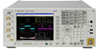
MXA Sep 06 X-Series Mid-performance 20 Hz to 26.5 GHz
